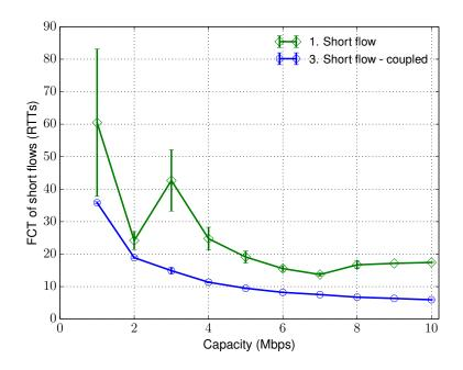
Flow completion time (FCT) of a short flow, with and without ctrlTCP
